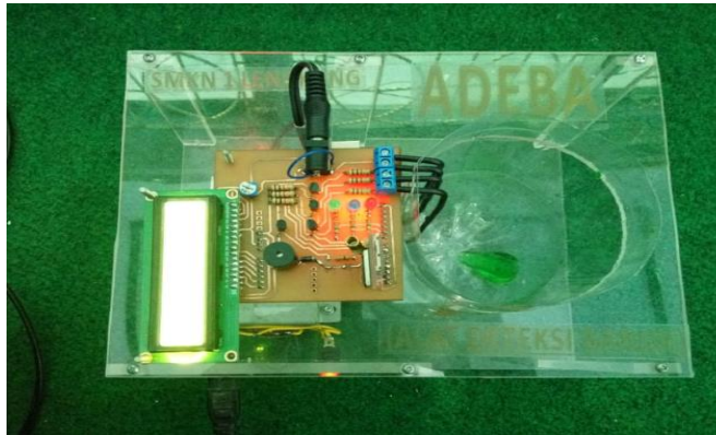
Gambar 1 ADEBA (Alat Deteksi Banjir)
